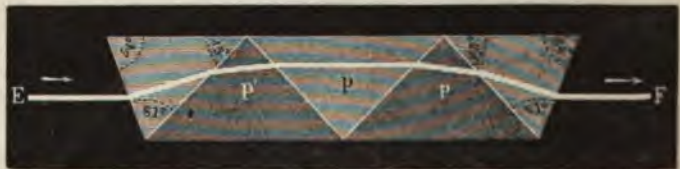
FIG. 54.—Direct-vision prism with five prisms.
